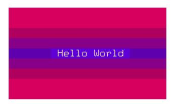
This program displays the string Hello World in the center of the screen. It uses a number of 256-color-mode colors to decorate the text, and will work in any terminal that supports 256-color mode. It will exit when Q is pressed.
